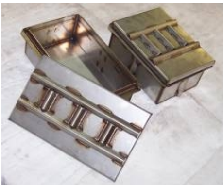
Alloy heat-treating boxes for use in the upper heating chamber
