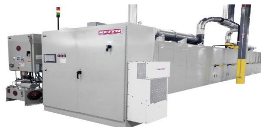
Pusher Kiln for calcining
