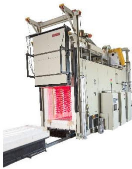
Envelope Kiln with pre-heater and thermal oxidizer
