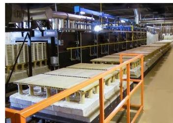
Gas Fired Car Tunnel Kiln for tile
